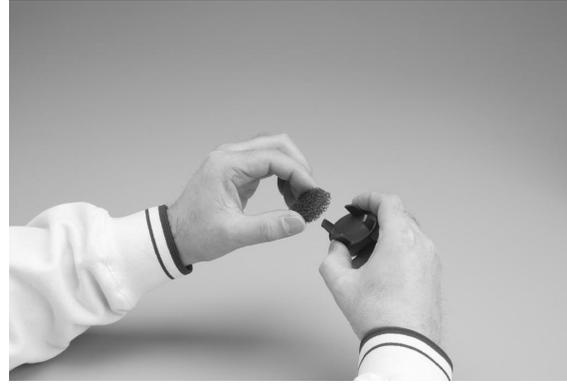
Figure 14: Removal of Filter from Filter Cover
